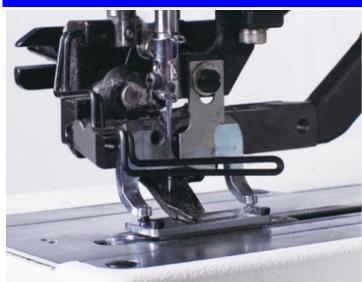
The HIKARI electronic straight button holer is equipped with a flexible cutting device, to cut as long as maximum 120 mm long buttonhole with just one knife mounted. The length of the mounted cutting knife is set up in the controller of the machine, and the computer calculates the number of cuts need to cover the length of the adjusted buttonhole. HIKARI supplies different length of knives for the machine from 6.4 mm to 31.8 mm in case a single cut is required by the technical specification.
