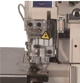
The LED light is built over the working area, together with the manual chain cutter switch. It is integrated to the machine head for better clearance of the movements of the operator. The LED unit is equipped with 9 LEDs, and it is adjustable in 9 levels to work easier with reflective materials.
