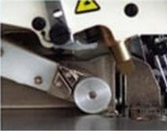
With the built in puller it is available to set up the feed of the fabrics with better accuracy. It is possible to adjust electronically the timing and the duration of the puller operations, at the beginning and at the end of the sew process, and mechanically the push force and the speed of the puller compared to the differential feed device. This system even allows to stretch the fabrics in case it is needed.
