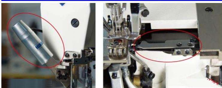
The HIKARI innovative direct drive flat bed interlock equipped with a stable and reliable upper and lower thread trimmer. With this feature we can greatly increase production efficiency and make the working conditions for the operator better.
