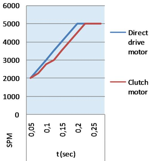
The direct drive sewing machines does not have transmission loss like the clutch motor machines. (The belt-drive sewing machine with servo motor has the same transmission loss as well. The increase of the production is about 14,6%. The belt-drive sewing machine sews 1000 meters. Under the same circumstances, the direct-drive sewing machine sews 1146 meters- in every shift.
