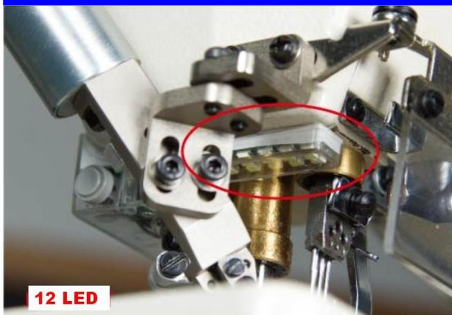
The HIKARI innovative direct drive flat bed interlock machine has built in the machine head LED lights. It is mounted to the machine head for better clearance of the movements of the operator. The LED unit is equipped with 12 LEDs, and it is adjustable in 4 levels to work easier with reflective materials, and provides better visualization for the operator.
