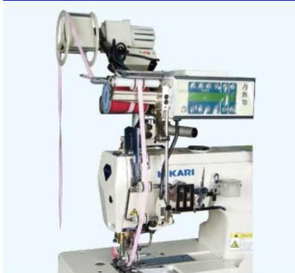
For the HIKARI innovative direct drive flat bed interlock the customer can order an optional computer controlled automatic feed device. Thanks for the computer control, the machine feeds the lace automatically. Depending on the needs of the operator the speed of the feeding is adjustable and the tension of the lace also.
