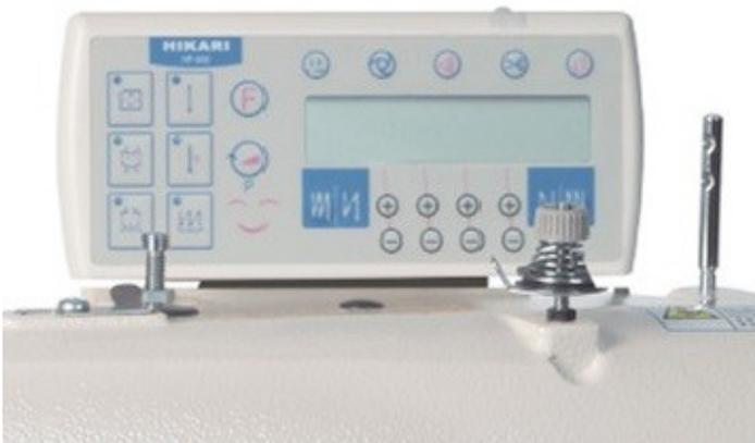
Full computerized, easy to use, user friendly control panel. The functions are grouped, and distributed according to the needs of the operator. The position of the functions are clearly separated, which helps the operator to use it faster to save time, and increase the efficiency. Functions like straight line and cycled sewing, backstitching, needle positioning, sewing speed and a other functions can be set up with the help of the LCD screen.
