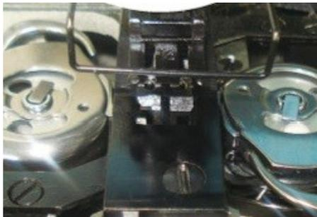
HIKARI redesigned the flexible straight knife thread trimmer system, to improve the flexibility of the double needle lockstitch machines in production. The system is equipped with easy to exchange larger capacity bobbins to achieve better efficiency. The machine is equipped with a standard 6.4 mm needle gauge set, and HIKARI offers a wide variety of gauge conversion sets from 3.2 mm to 25,4 mm for both normal and heavy duty machine variants.
