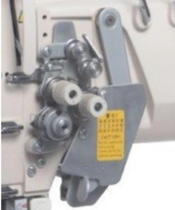
During normal production both of the needle bars are working. In case the operator would like to form a corner, each of the needle bars can be switched off with the quick split needle bar actuation switch, which is placed on the front side of the machine.
