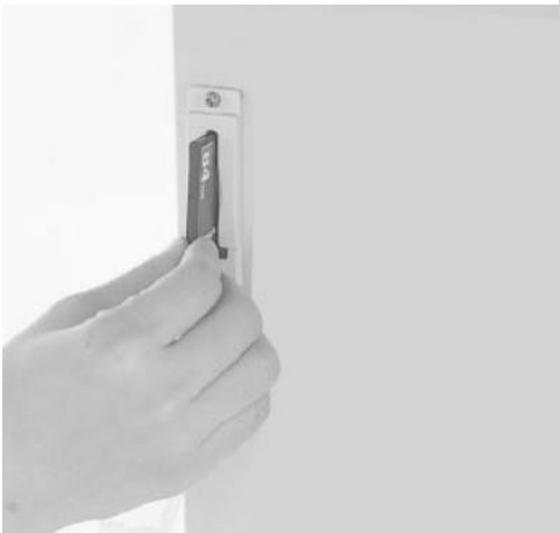
On the HIKARI innovative pattern sewing machine there are two ways to upload your patterns, with a CF memory card through the CF memory card reader which you can find under the machine, or with the optional pattern editor, which we can use to write our own patterns and we can upload them to the built in CF card reader.
