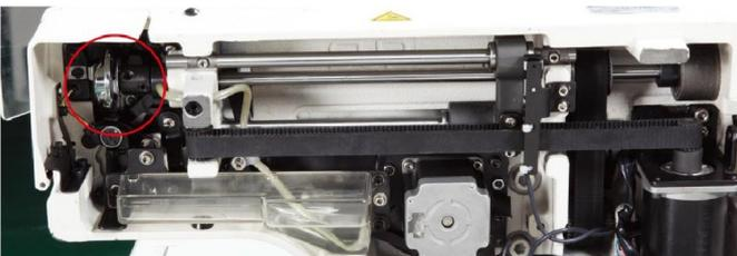
The machine is equipped with a central lubrication system, which offers as minimum oil leaks on the garments as possible. The oil is placed in a central reserve, and has been pumped to the contact place on small diameter pipelines and wicks. The lubrication monitoring gauge is installed on the side of the machine which is easy to observe.
