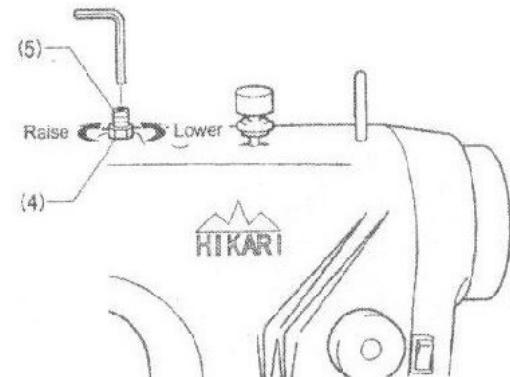
Easy to adjust, micro lift function to lift the presser foot from 0,1 to 4 mm to the needle plate. These properties together, with the stitch length, and the flexible trim gives a unique machine for the production.
