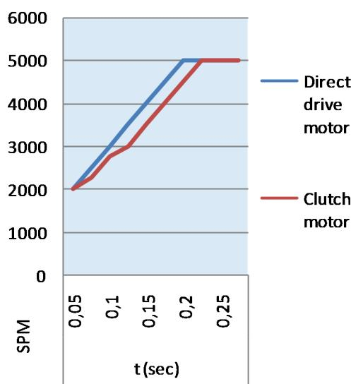
The direct drive sewing machines does not have transmission loss like the clutch motor machines. (The belt-drive sewing machine with servo motor has the same transmission loss as well. The increase of the production is about 14,6%. The belt-drive sewing machine sews 1000 meters. Under the same circumstances, the direct-drive sewing machine sews 1146 meters- in every shift.
