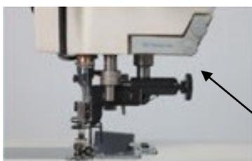
The LED light is built together with the reverse switch. It is integrated to the machine head for better clearance of the movements of the operator. The LED unit is equipped with 10 LEDs, and it is adjustable in 5 levels to work easier with reflective materials.
