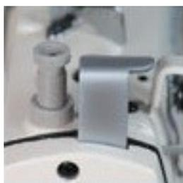
The built-in edge cutter, is an on demand cutter, which is possible to switch on and off in case it is needed. If the cutter is switched off, the machine can be used as a regular single needle lockstitch machine.
